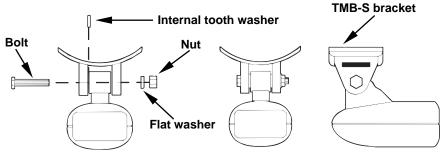
Attach motor mounting bracket to transducer.
